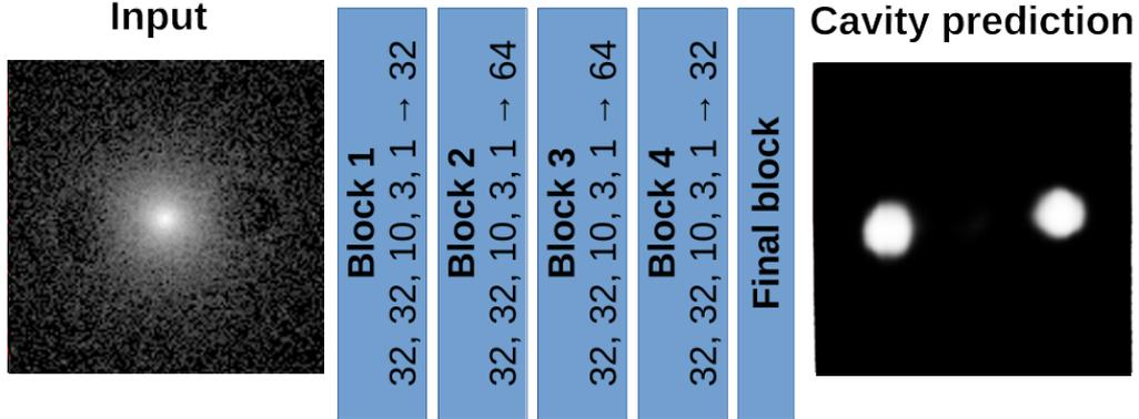
Figure 3.2: A diagram of the used architecture. An input image is fed into a sequence of 4 convolutional blocks, each containing presented number of filters. Afterwards follows the final layer (see text for details). The output is a pixel-wise cavity prediction where white indicates a high level of confidence that cavity is present. Batch norms and ReLUs are omitted for clarity. The figure was adapted from Fort (2017), modified.
