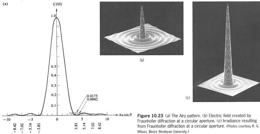
**Figure 10.23** (a) The Airy pattern. (b) Electric field created by Fraunhofer diffraction at a circular aperture. (c) Irradiance resulting from Fraunhofer diffraction at a circular aperture. (Photos courtesy R. G. Wilson, Illinois Wesleyan University.)
