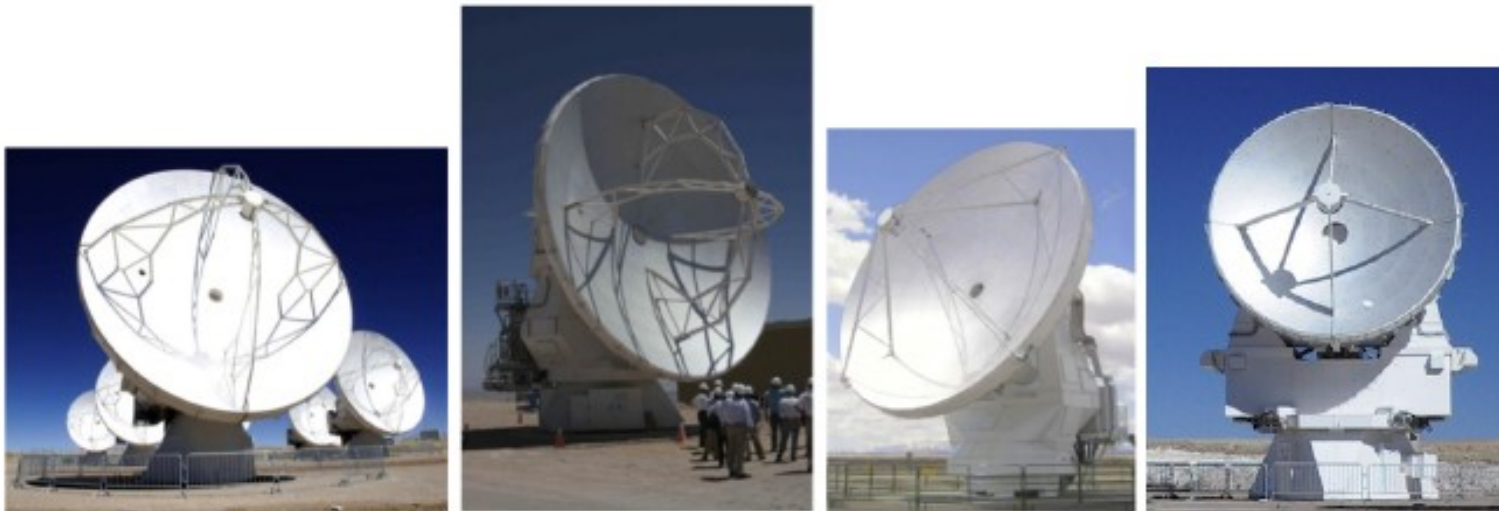
Figure A.1: The four different ALMA Antenna designs: Vertex 12 m, MELCO 12 m, AEM 12 m, and MELCO 7 m (from left to right).
