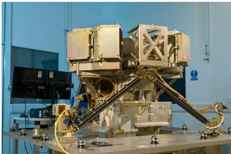
**Fine Guidance Sensor and Near Infrared Imager and Slitless Spectrograph (FGS-NIRISS)** 0,8 až 5  $\mu\text{m}$
